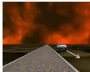
Approaching situation. Path of the second car was parallel to the lane. Speed of both the driver's car and the approaching car was 20 m/s.
